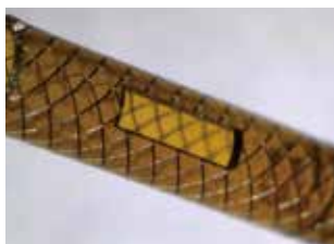
Single process on a hybrid material. (Polyamide, polyimide, and stainless steel wire)
