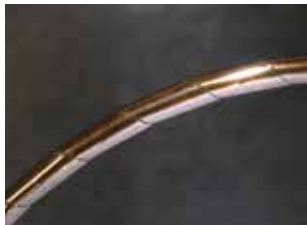
Spiral grooves on a polyimide tube. I.D.: 1 mm, thickness: 0.06 mm
