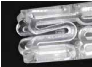
Cutting on a polylactic-acid tube. O.D.: 1.52 mm, I.D.: 1.09 mm
