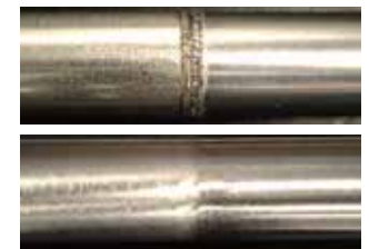
NiTi, an intermediate material, and stainless steel are welded together. (The photo below shows a tube applied a simple finishing)
