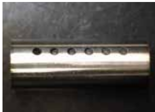
Dimple forming on a NiTi tube. Dimple depth from the left : (through) 0.5, 0.4, 0.3, 0.2, 0.1, 0.05 mm
