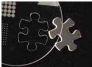
Cutting on a sapphire glass sheet with 0.8 mm thick.
