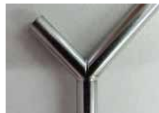
Y-shaped pipe with thin wall thickness. (pipe dia. 2.4 mm, thickness 0.25 mm)
