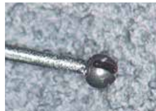
Spot welding for dia. 0.3 mm stainless steel ball with dia. 0.08 mm stainless steel wire
